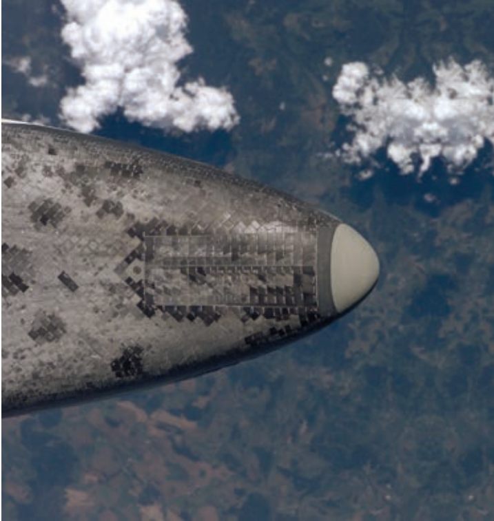
Space shuttle ceramic heat protection shield
